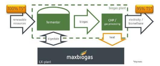
The easiest application is the pre-treatment of biogas digestate. The solid parts of the digestate are mainly composed of cellulose und hemicelluloses which were not available for biogas production. The maxbiogas LX-plant pre-treats the digestate in such a way that it is transformed almost completely into biogas in the biogas plant fermenter. The energy used by the maxbiogas process is supplied by the power generation or by the gas purification of the biogas plant.
